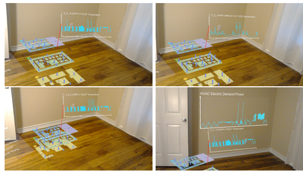
Figure 10. Interactive exploration of building attributes and movement patterns from employees for investigating event correlations. The four examples demonstrate that a user can select and visualizes four attributes respectively: F2 Z15 Supply Inlet Temperature, F2 Z14 Return Outlet CO2, F1 Z5 Supply Inlet Temperature, HVAC Electric Demand Power.
