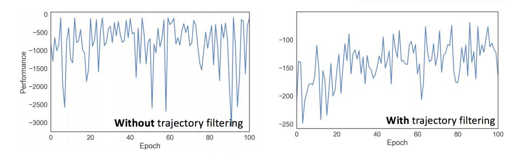
The training curves of RLScheduler on PIK-IPLEX2009 job trace with and without trajectory filtering.
