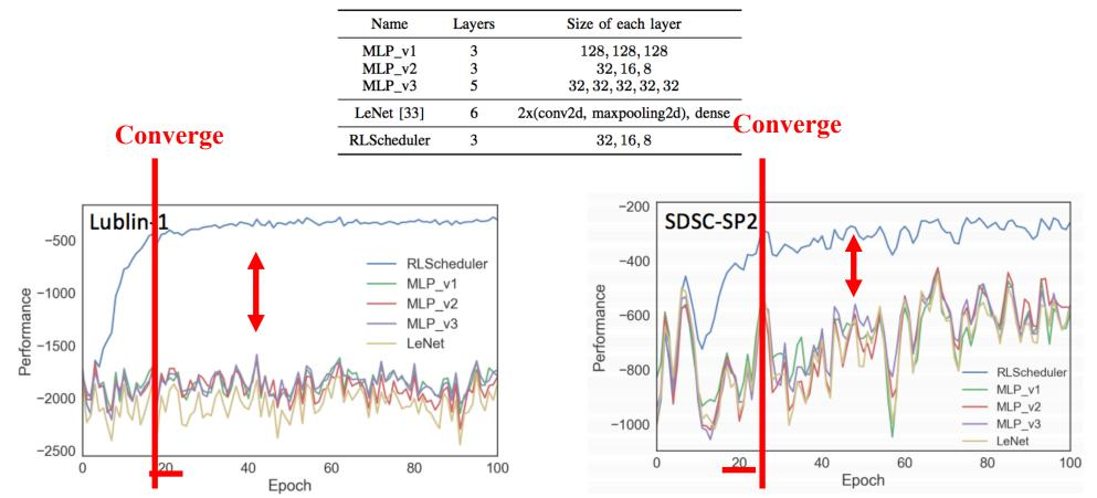
The horizontal axis shows the total number of training epoch; the vertical axis shows the performance of the agent. The larger vertical axis value indicates a smaller average bounded job slowdown and is better
