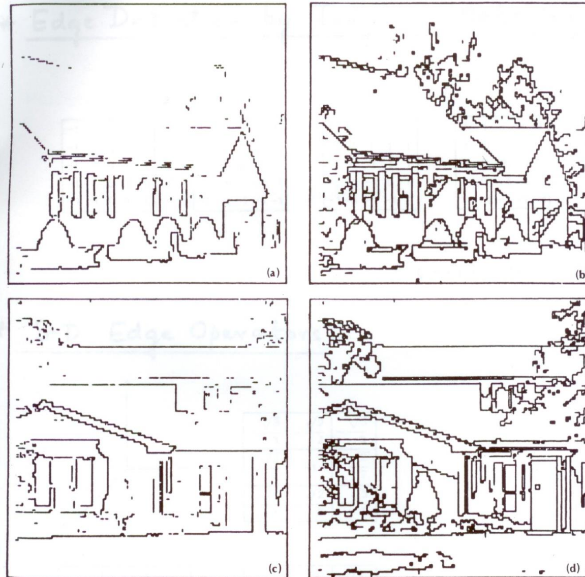
Fig. 3.22 Edge relaxation results. (a) Raw edge data. Edge strengths have been thresholded at 0.25 for display purposes only. (b) Results after five iterations of relaxation applied to (a). (c) Different version of (a). Edge strengths have been thresholded at 0.25 for display purposes only. (d) Results after five iterations of relaxation applied to (c).
