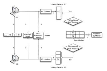
Figure 1. Control Flow Graph of VIAF
