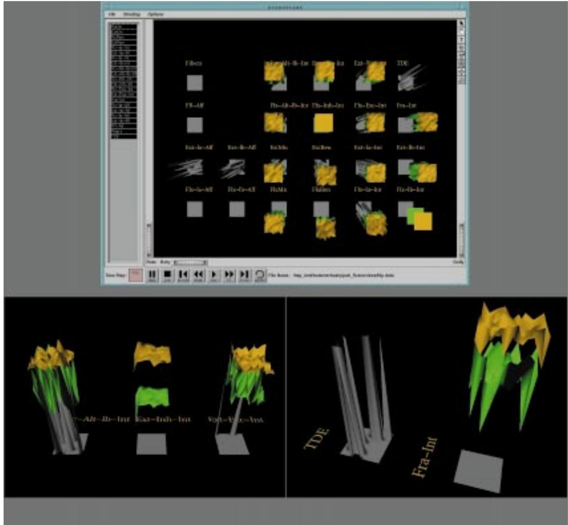
resented. Each variable appears as a height field. Thus, as the function values change over the grid, the quad mesh vertices are proportionally scaled to reflect the changes in the function. The field values directly determine the amounts by which the membrane potential and threshold fields are raised (no additional scaling is performed), while the spike field is scaled by a user-defined value.
