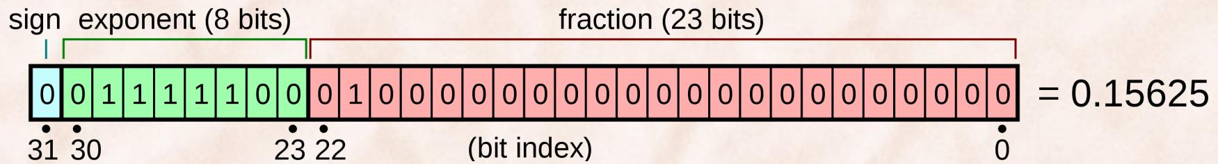
$$\text{value} = (-1)^{\text{sign}} \times 2^{(E-127)} \times \left( 1 + \sum_{i=1}^{23} b_{23-i} 2^{-i} \right).$$
