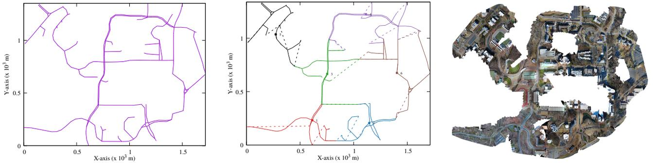
Fig. 1. Line coverage of a road network graph by multiple UAVs. (left) A map of the UNC Charlotte campus. (middle) The graph is clustered into smaller components, each represented by a different color. The generated tours for UAVs covering the graph are shown, with dashed segments indicating deadheading travel. (right) An orthomosaic of the road network computed from photos taken by the UAVs flown autonomously along the generated tours.
