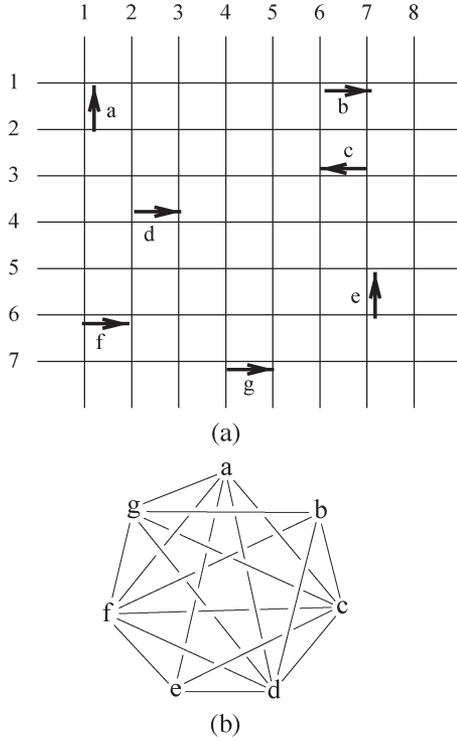
Fig. 13. (a) Grid of control wires indicating droplets with horizontal and vertical movements. (b) Corresponding transition graph for droplet movements.
