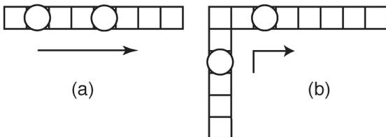
Fig. 11. Minimum number of empty cells between two occupied cells to ensure that the droplets cannot combine or split inadvertently depends on the path shape. (a) When the two cells are on a straight line. (b) When the two cells are around a bend in the path.
