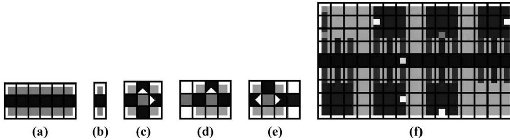
Fig. 3. Components. (a) A street. (b) A connector component. (c) An intersection. (d) A source connected to an intersection. (e) A sink connected to an intersection. (f) An active work area, showing several mixing units with droplets (depicted as small squares).
