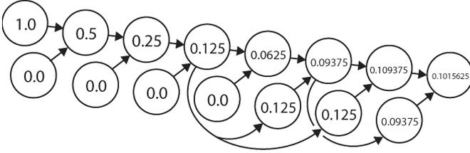
Fig. 15. An example mixing graph for dilution control. The scheme assumes that droplets of a specified concentration level are given and that buffer droplets of 0% concentration are available. Any desired reduced concentration can be achieved; our approach is to identify the intermediate droplet concentrations through a binary search strategy. Here, the concentration is reduced to approximately 10% of its original level.
