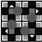
Fig. 9. When droplets are in this particular configuration, they cannot move again. Attempting to advance any droplet would require activating the adjacent electrode, which is also diagonally adjacent to another droplet. This activation could result in unexpected droplet movement or mixing, and therefore, is disallowed.
