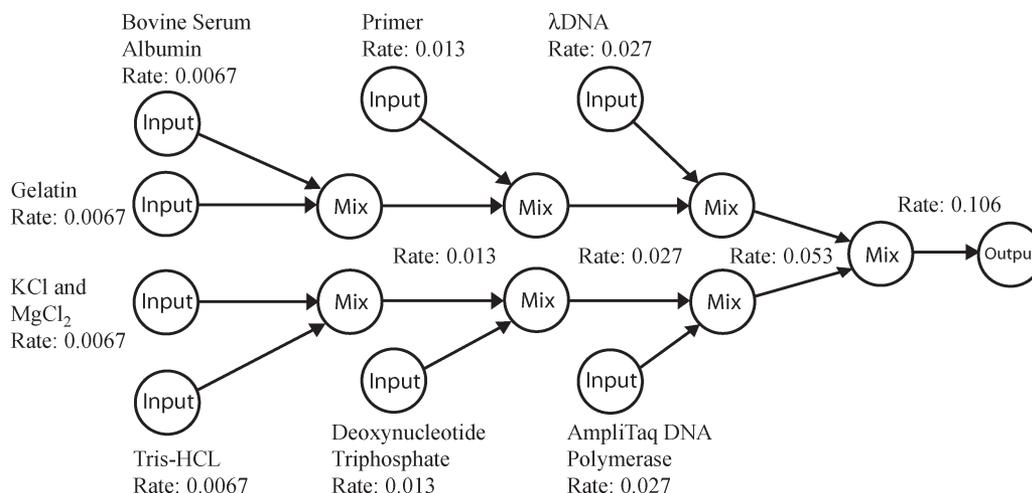
Fig. 6. PCR analysis graph. Input nodes are labeled with the samples they introduce and the rate at which they introduce them, in droplets per cycle. Edges out of mix nodes are labeled with the droplet rate resulting from the operation.
