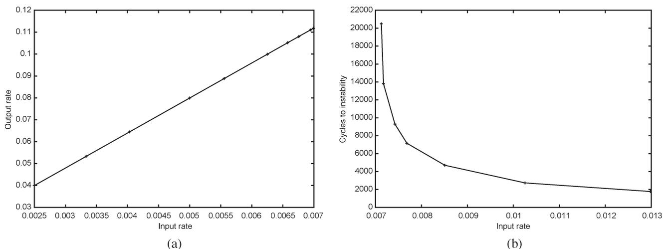
Fig. 7. Simulation data for the PCR analysis illustrating (a) variation of droplet output rate with input rate in the stable range, and (b) number of cycles at which the system goes into deadlock, as input rate is increased in the unstable range. For this example, mixing time is 128 cycles, the number of mixing units per work area is 8, and the tiles are in a  $2 \times 2$  pattern.
