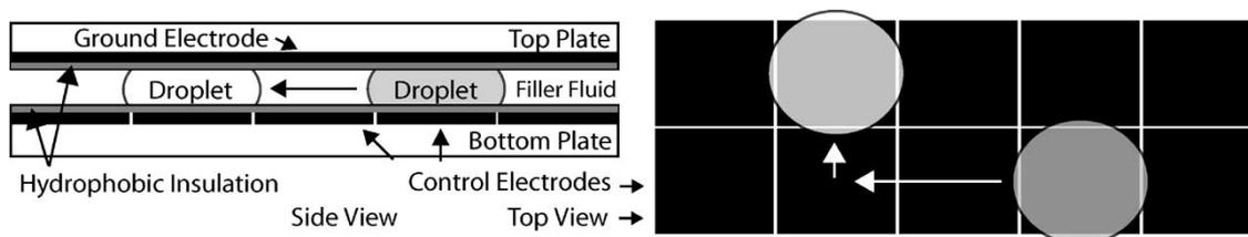
Fig. 1. Droplets on an electrowetting array (side and top views). A droplet moves to a neighboring control electrode when the electrode is turned on. The electrode is turned off when the droplet completes its motion. Based on [29].
