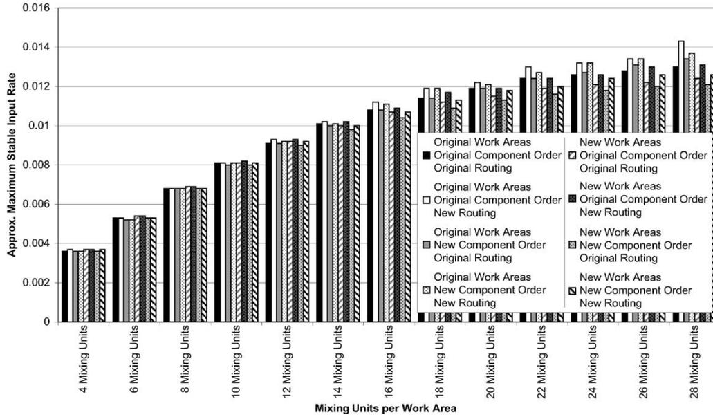
Fig. 10. Chart depicting the effects of each of the three routing-control variations on a 2 × 2-tile PCR simulation. Input rate is measured in droplets per clock cycle. Each bar in the graph corresponds to operating the system under a certain set of parameters. Parameters labeled as “new” correspond to the new methods in Section IV-B. Parameters labeled as “original” correspond to the original methods described in Section III.
