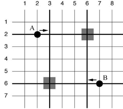
Fig. 14. Small grid of control wires with two droplets to be moved. Droplet A must move to the right and droplet B must move to the left. Actuating them simultaneously will also activate the electrodes marked with gray squares. If these electrodes cause undesired droplet movement, then droplets A and B interfere with each other.
