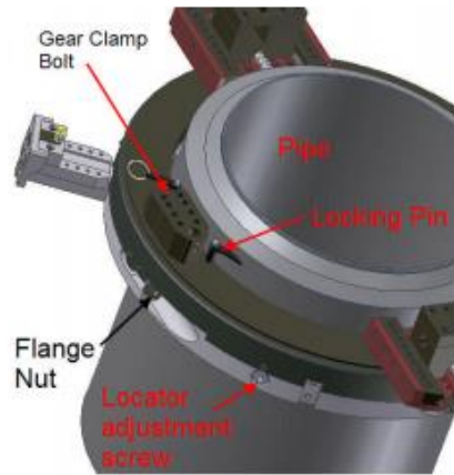
Figure 17: Clamshell Lathe Attaching to the Proposed Canister
