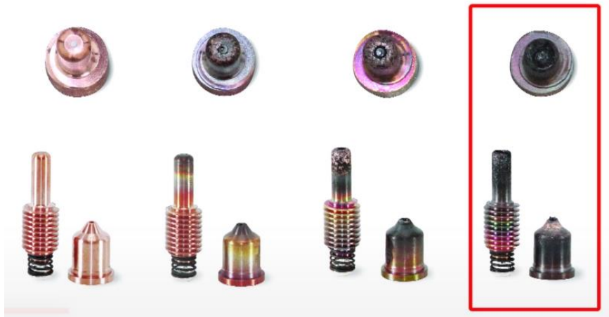
Figure 31: Nozzle and Electrode Consumables for Plasma Systems
