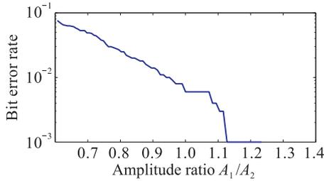
**Fig. 5** The BER value with respect to amplitude. The x-axis is the ratio of amplitude between two sequences.
