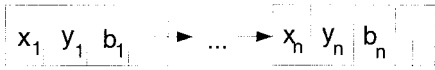
Fig. 2. A linked list chromosome representing a path. Each node contains x and y coordinates of a point together with a state variable b , which provides information on feasibility of the point and the following path segment. The point (x_1, y_1) is the starting point, and the point (x_n, y_n) is the goal point.
