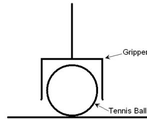
(a) Pick-up and put-down end-effector configuration
