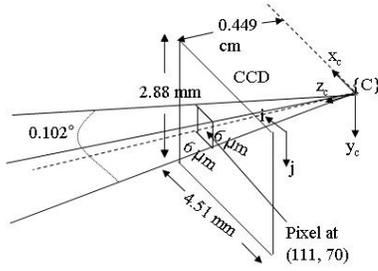
Fig. 8. Dimension of atomic obstacles as defined by the CCD of the camera for resolution  $752 \times 480$
