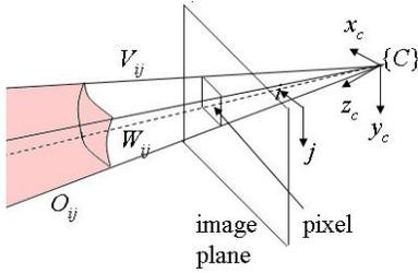
Fig. 1. The geometry of an atomic obstacle  $O_{ij}$  from a stereo vision sensor
