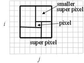
Fig. 6. Division of a super pixel into one pixel and four smaller super pixels
