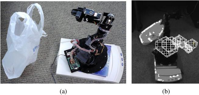
Fig. 9. (a) Testing environment, (b) Stereo vision image at  $\tau_0 = 0$ (s) and for the CT-point  $\chi_1$ , with the partitioned projection image  $P(E)$  of the robot's dynamic envelope  $E(\chi_1, \tau_0)$ .
