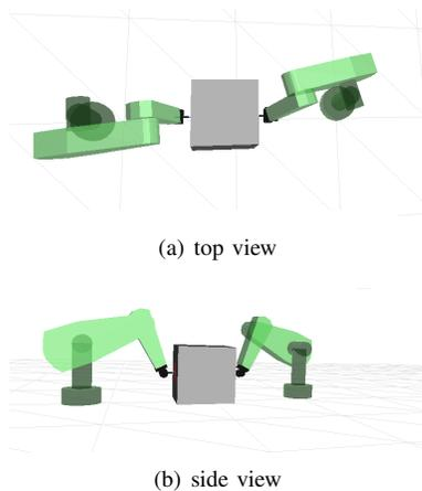
Fig. 1. Two grasping configurations for the two robots
