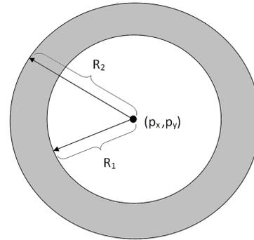
Fig. 3. Valid base region for end-effector position  $(p_x, p_y, p_z)$  given by radii  $R_1$  and  $R_2$
