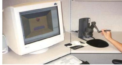
Fig. 11: Haptic interaction via a PHANToM Desktop
