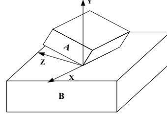
Fig. 2: An example task frame with respect to a line PC
