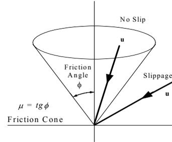
Fig. 9: Static Friction Cone
