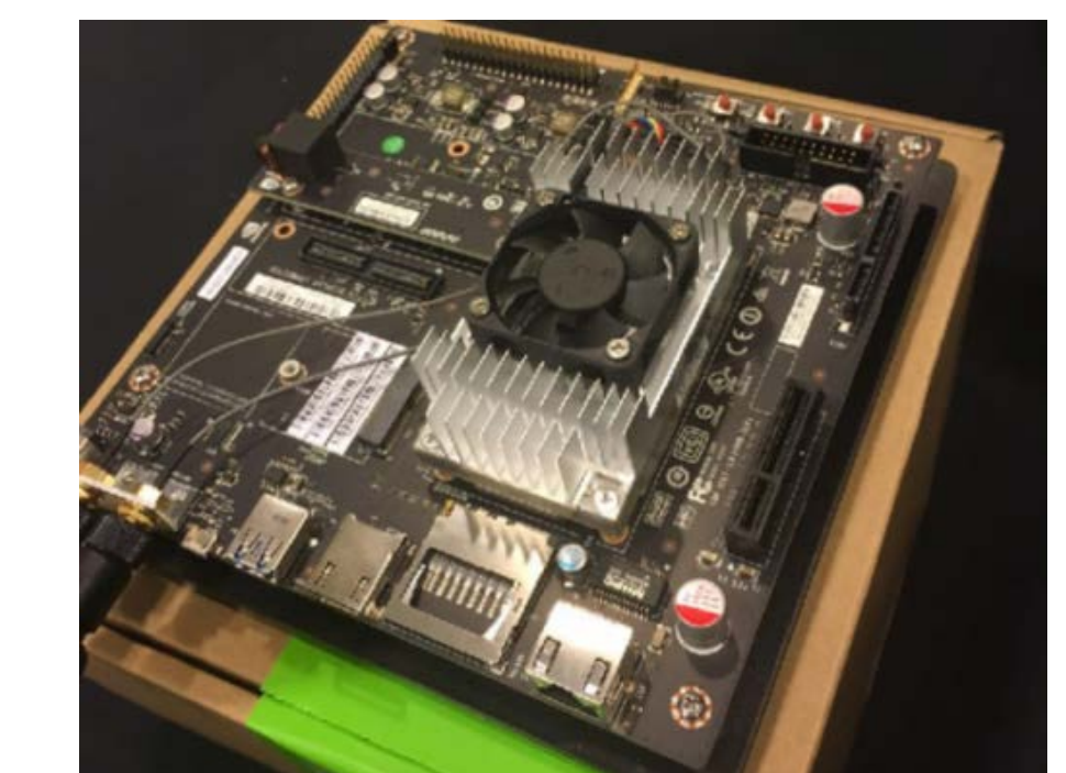
NVIDIA TX1. 64-bit, ARM Cortex A-57 (big.LITTLE architecture)
