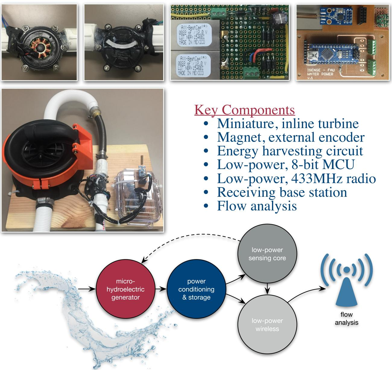
Even at modest flow rates, well below those observed in typical household irrigation systems, continuous operation is possible.
