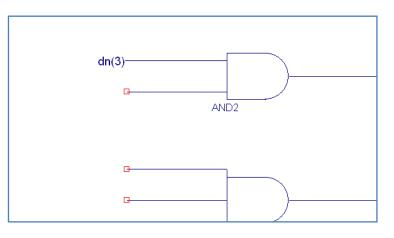
• Continue with this process, of naming wires, until all the wires are named as shown in the following figure. *Note:* there are d(x) and dn(x). Also, note that the output is named "prime".
