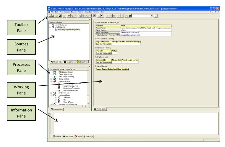
• Double click on the primeDet\_top.sch item in the Sources pane. An empty schematic sheet will open in the Working pane.
