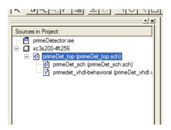
• Making a model then placing it into a schematic is referred to as a Hierarchical structure. You can nest models as deep as you please. The idea is to break the design into manageable pieces.
