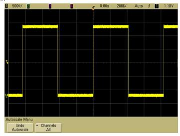
à When we connect a probe that can be calibrated the **Calibrate probe Softkey** will be active then connecting the probe in the probe comp terminal will help us to calibrate the probes.
