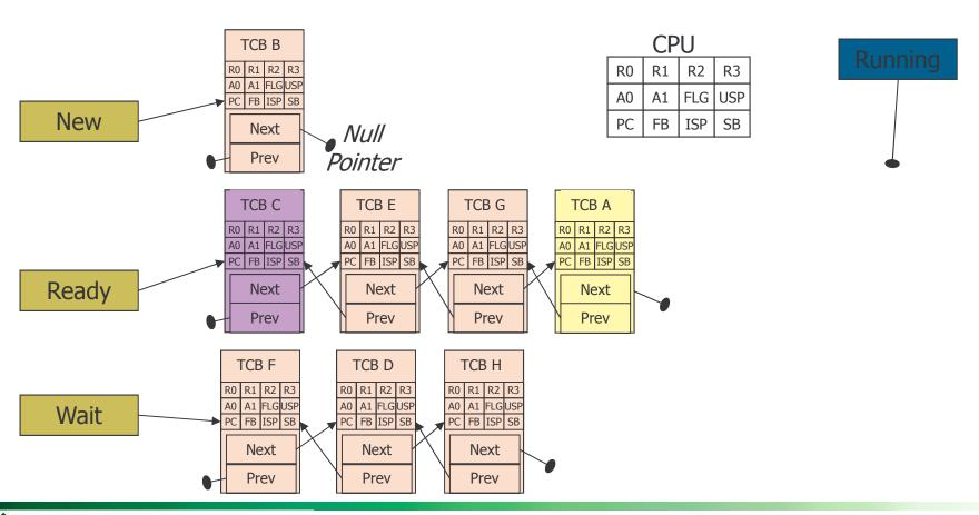
Remove thread C from the ready queue and mark it as the thread to run next
