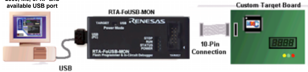
Figure 1 ICD System Connectivity
