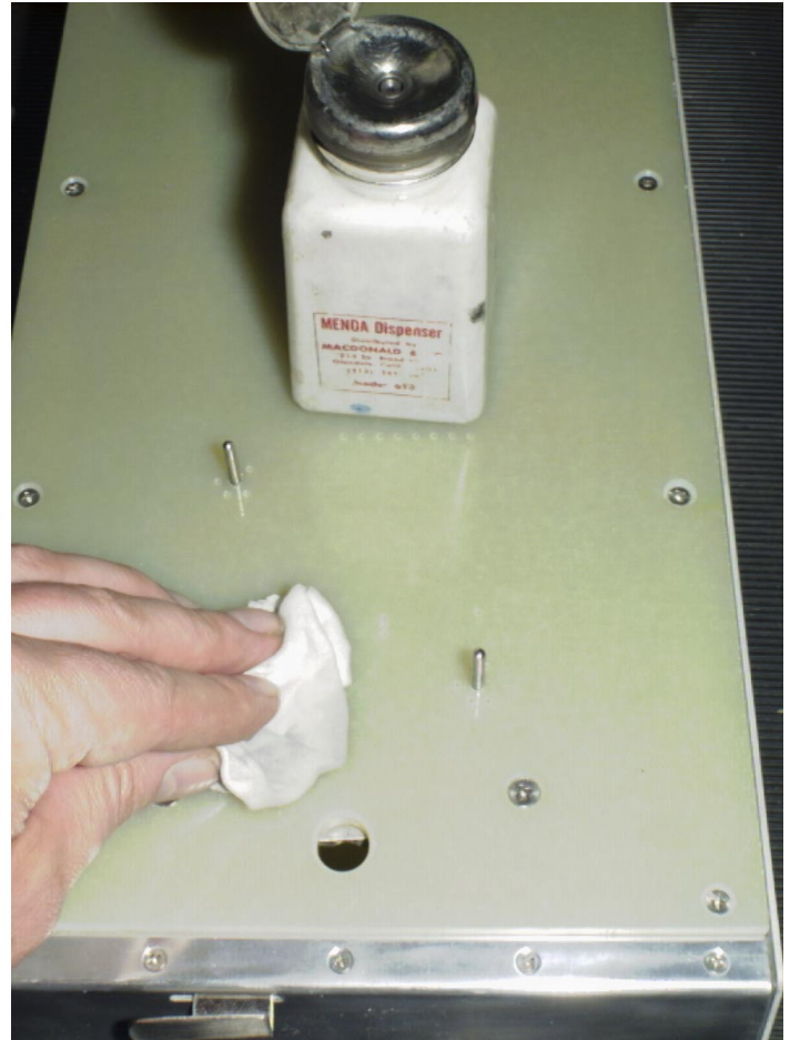
Wipe excess adhesive off with isopropyl alcohol
