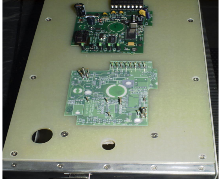
Finished Bed of Nails Plate.
