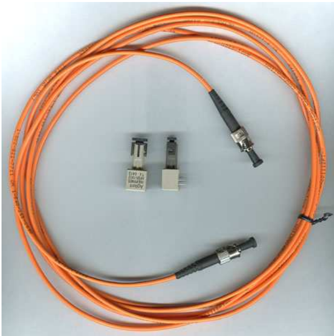
FIGURE 1 FIBER OPTIC CABLE AND TRANSMISSION DEVICES
