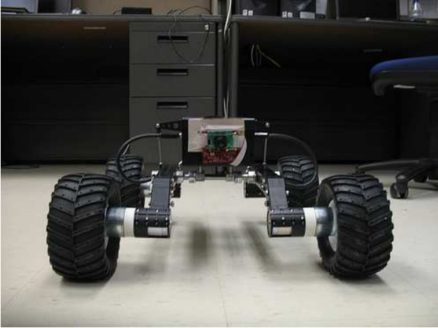
Figure 2: Vehicle platform with CMUcam3 without screen
