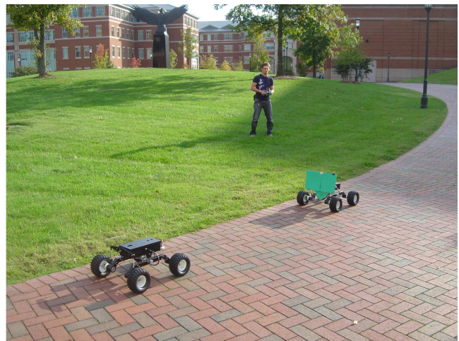
Figure 3: Example of autonomous vehicle with CMUcam3 following a remotely controlled vehicle with a colored card.
