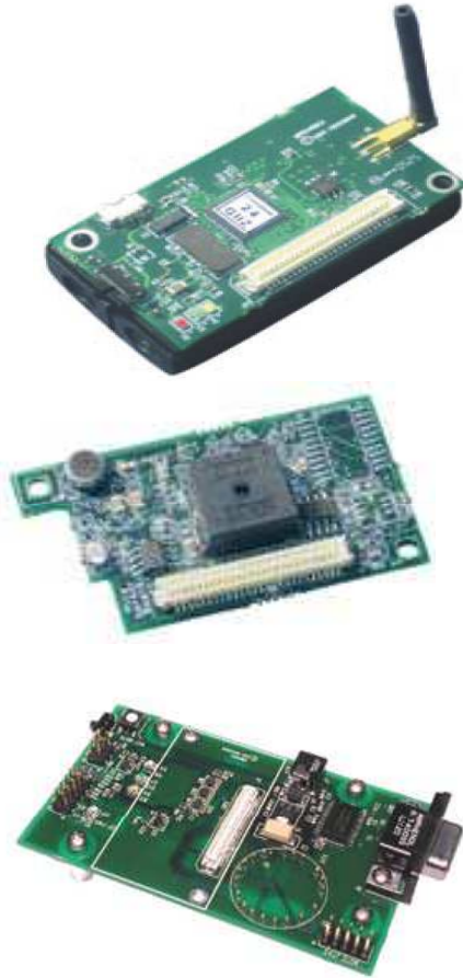
Figure 1: Crossbow products used [2]: (a) MICAz mote, (b) MTS300 basic integrated sensor board and (c) MIB510 interface board
