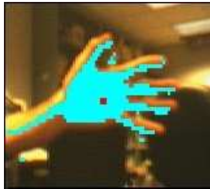
Figure 3: Example hand image captured by the graphical user interface with tracked bitmap (light turquoise) and centroid (dark red dot) overlaid.
