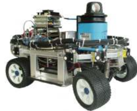
Figure 2. Autonomous vehicle equipped with the SICK LD laser scanner, ultrasonic sensor cells and the PC-104 system.
