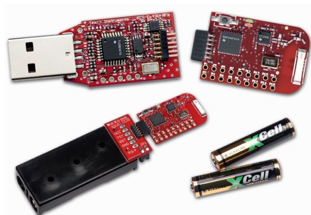
Fig. 10b: TI eZ430-RF2500 development kit 6
