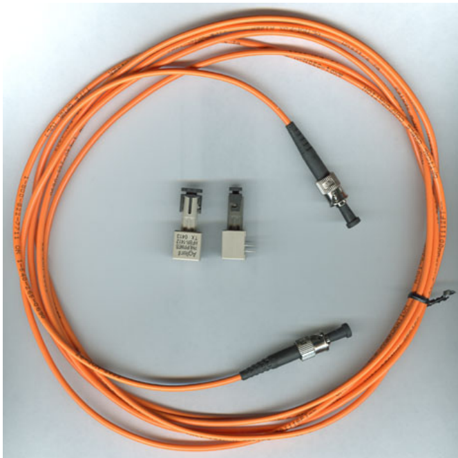
FIGURE 1 FIBER OPTIC CABLE AND TRANSMISSION DEVICES
