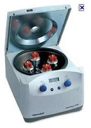
Set speed (note rotor and tube limits) Balance tubes: 2 tubes with the same mass are 180° from each other Set speed Set temperature Set rate
