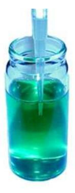
To aspirate the sample into the tip, allow the pushbutton to return slowly and smoothly to the fully extended UP POSITION.
