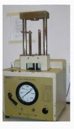
HydroShear is an example of point-sink-shearing: is uses a high-pressure LC pump to shove DNA through narrow tubing.
