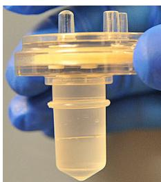
10. Immediately before installation on the Ion OneTouch™ Instrument, *slowly* invert the Reaction Filter and Reaction Tube assembly to this position. Do **not** mix the Oil and amplification solution.
