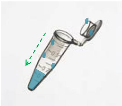
Denser material will collect at the bottom of the tube.
