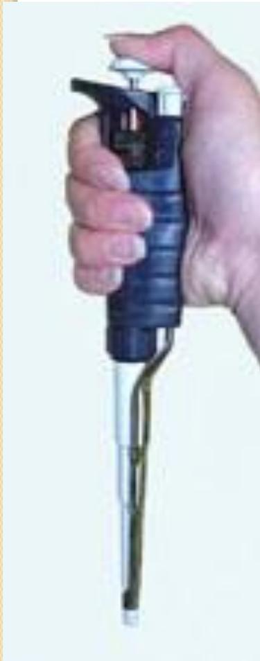
*Depress the plunger first: don't put the tip in the liquid and then depress the plunger (the pressure is different).*
