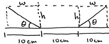
gutter formed by bending the meter sheet in thirds
