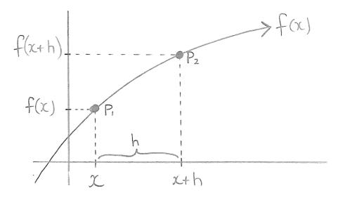
In order to get the two points  $P_1$  and  $P_2$  as close together as possible, we need for the space  $h \rightarrow 0$ . So, the slope between  $P_1$  and  $P_2$  is:
