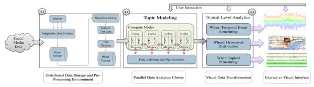
Figure 4: An overview of I-SI architecture. There are 4 major components in the I-SI architecture: Distributed Data Storage and Pre-Processing (Section 4.1), Parallel Data Analytics Cluster (Section 4.2); Visual Data Transformation; Interactive Visual Interface (Sec. 4.3).
