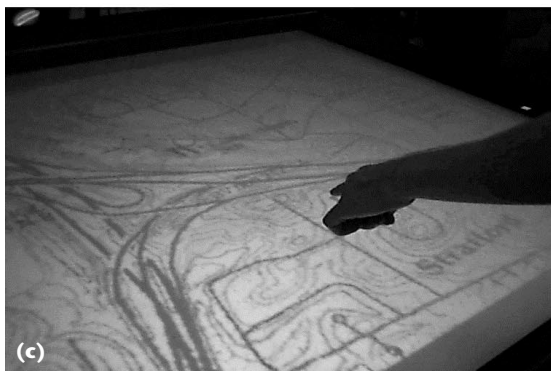
14 Terrain navigation using deictic gestures: (a) panning, (b) rotating (about an axis perpendicular to and through the end of the rotation lever), and (c) zooming.
